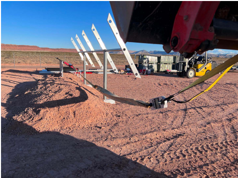
PHOTO 3: Horizontal force test setup
