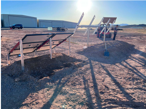
PHOTO 2: Horizontal force test setup
