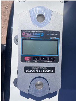
PHOTO 1: Dynamometer used to record loads
