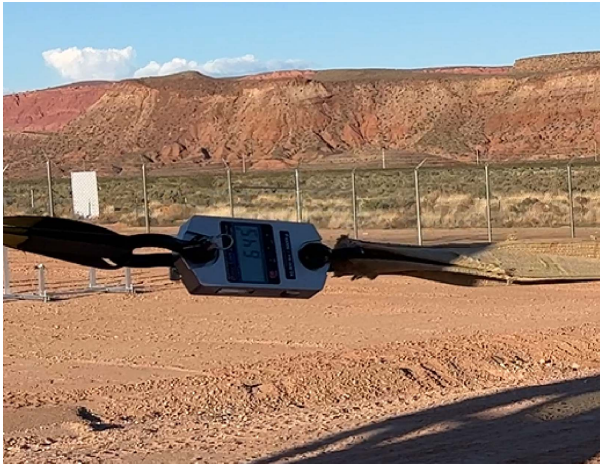
Photo 4: Horizontal force test max load
