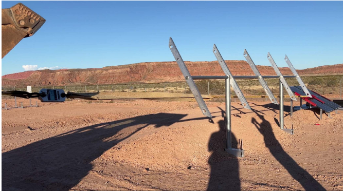
Photo 4: Horizontal force test at max load
