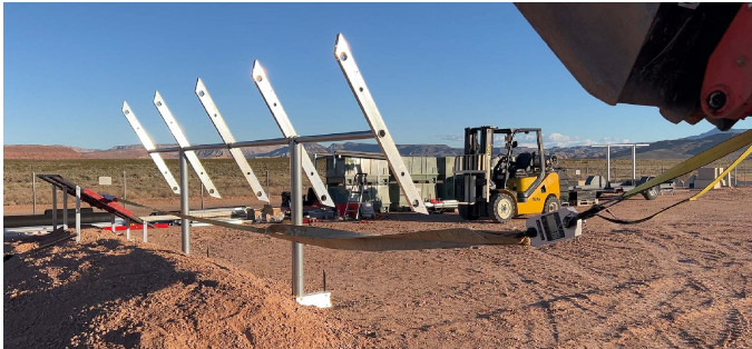
PHOTO 1: Horizontal force test setup
