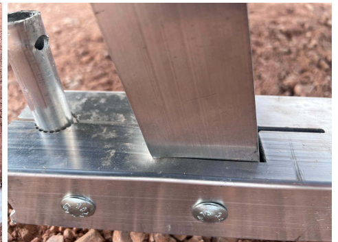
PHOTO 15: Upright deformation after testing
