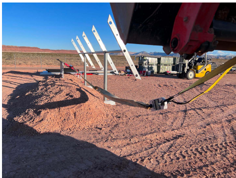
PHOTO 3: Horizontal force test setup
