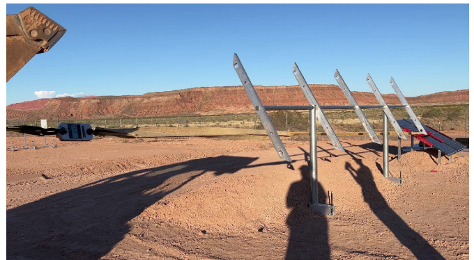
Photo 4: Horizontal force test at max load
