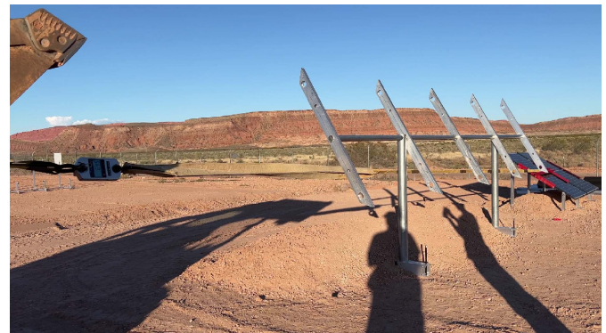
Photo 4: Horizontal force test at max load
