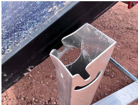
PHOTO 14: Upright mount deformation after testing
