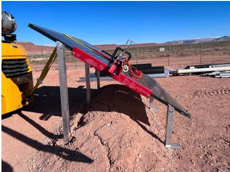
PHOTO 13: Ballast after completion of testing
