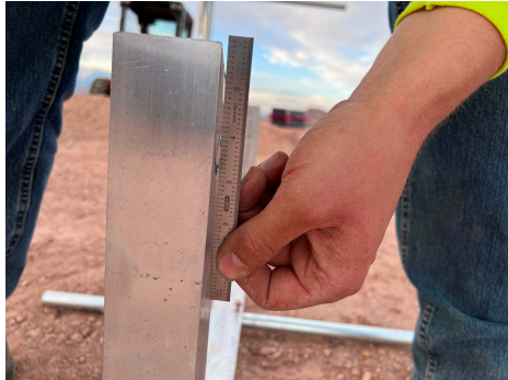
PHOTO 10: Slight deformation after load removed
