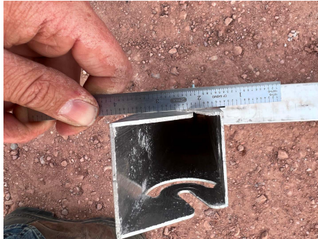
PHOTO 11: Slight deformation after load removed
